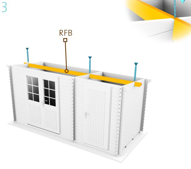
PLACE THE FIRST ROOFBOARD FLUSH WITH THE END OF THE PURLINS AND ATTACH WITH 6 SCREWS, 3 INTO EACH NEXT, SAW THE LAST BOARD TO MAKE IT FIT.
