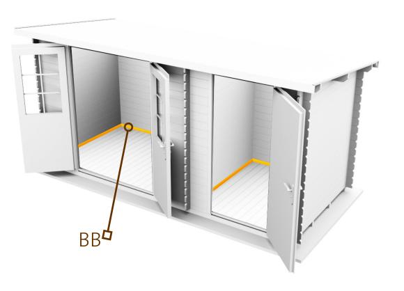
DRILL THROUGH THE WALL, HOLE MUST BE AT THE BOTTOM OF THE OVAL, ATTACH WITH BOLT.
